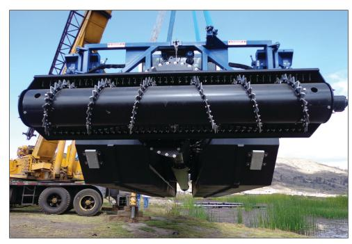
The Razor Tooth Weedmaster unit mounts directly to the pump inlet door. It measures 9 ft (2.7m) wide and consists of a steel shroud and cutterbar with dual direct drive motors driving the cutter. The cutterbar is constructed of heavy wall tubing with reinforced double edged razor teeth designed exclusively by IMS. The shroud contains two rows of static cutter blades that clean the main cutterbar as it rotates.
