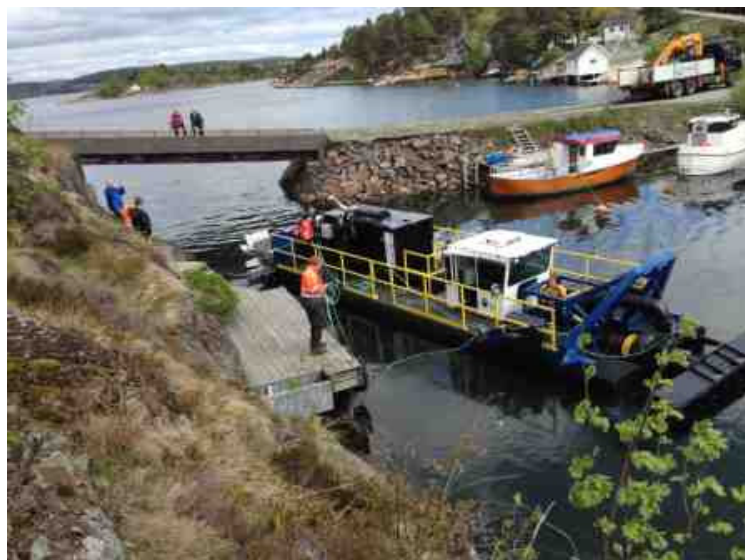
The 15.7m long, 3.7m wide 7012 HP Versi-Dredge fit snugly underneath an overpass that was just 2.3m at its highest point.
