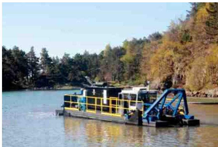
The 7012 HP can dredge berths down to 9.1m (30 ft.) depth and create an even bottom profile with no ridges due to its horizontal cutterhead design.
