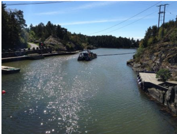
In a matter of just days the 7012 HP dredged an inlet/marina on Tromøy, pumping the hard shell sand to a dewatering site ½ km away.
